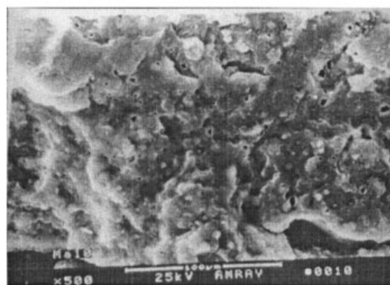
Figure 4 SEM micrographs of fracture surface of IFR/PP composites: (a) composite B; (b) composite C; (c) composite E.
